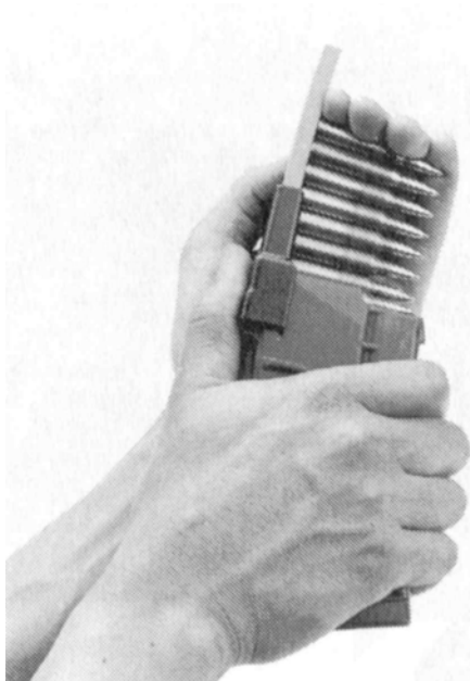
Loading the cartridges into the magazine by means of the loading tool
