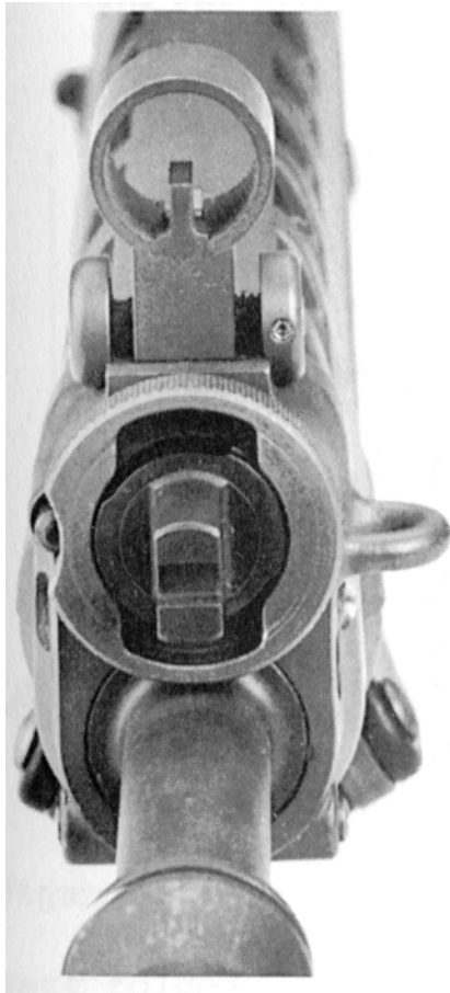
Gas valve in position I
